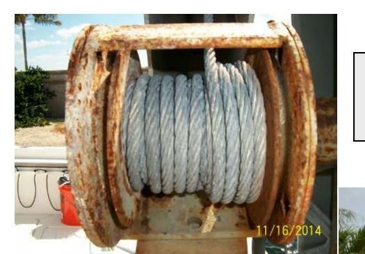
Galvanized lift cables are very susceptible to rusting. The cable on the left is still in good condition at the winder spool.
