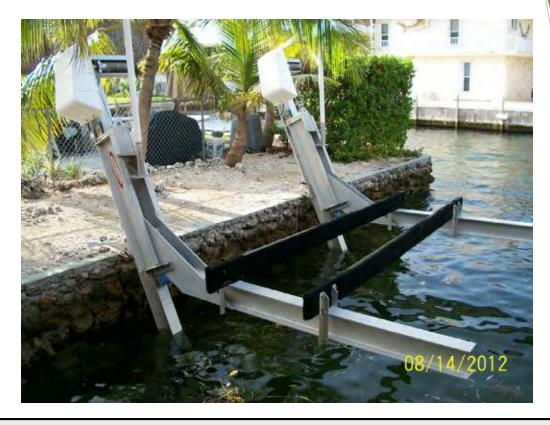
All side elevator boat lifts have metal components that are ALWAYS submerged in the water. When these in-water components deteriorate it can destroy a boat lift in a short period of time, especially if the lift is left plugged in to an electrical source. That is why ALL lifts that have in-water metal components MUST have sacrificial zinc anodes to protect the lift structure.
