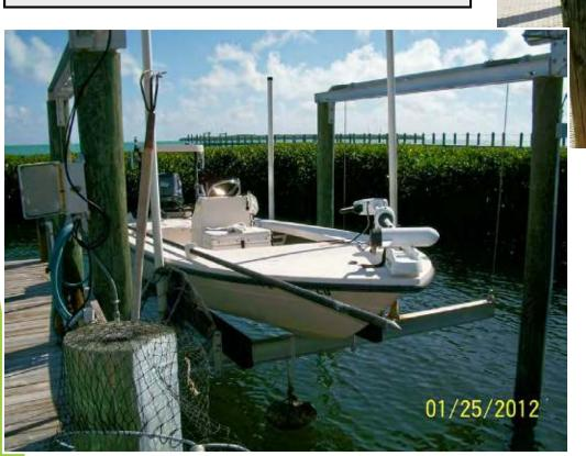
The greatest difficulty with these lifts is that most times you will not be able to inspect the outer beam components, unless you are brave enough to walk out on the bunks. Also, if there is a vessel on the lift it will restrict your access.
