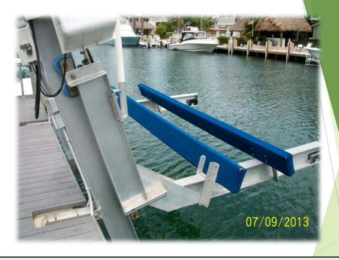
Side elevator lifts are like a forklift that have lift cables or hydraulic pistons. Side elevator lifts are very stable and can be designed for boats of all sizes up to 25,000 lbs. Side elevator lifts typically mount on the canal bottom and are stabilized with anchor plates to the dock surface.
