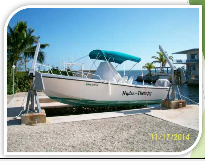
Davits are basically small cranes mounted on concrete bases or pilings that lift and support boats with cables. Davits can be belt-driven, direct chain driven or hand winched. Davits can be rated from 500 lbs to a maximum of 5,500 lbs per davit.
