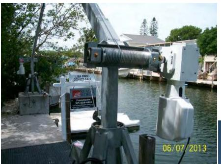
Direct gear drive motors are usually direct drive shaft or drive chain.
