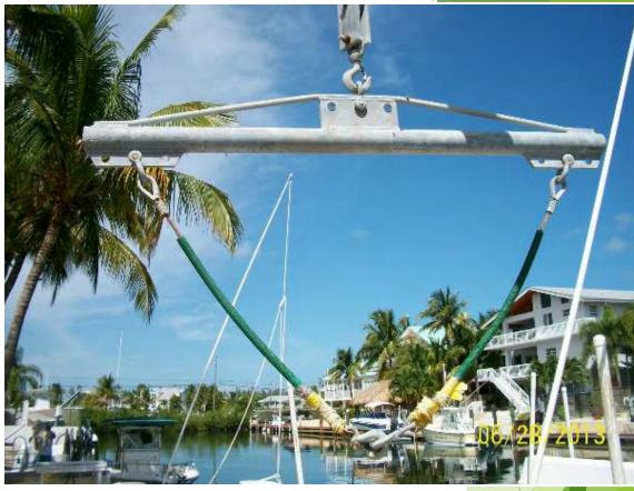
The stern spreader "T-bar" is a very important part of a davit inspection. The spreader bar is used at the stern of the boat to keep the weight of the boat even for stable lifting. Always look for the T-bar... many times they are not on property because they left with the previous owner or they have been stolen. Always document their presence or absence in your report. A new T-bar costs \$300.00
