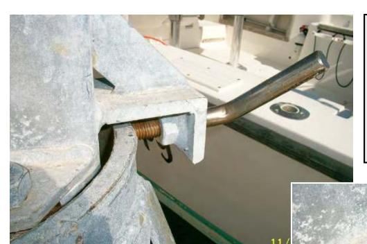
Inspect davit locking bolts for condition. If corroded, recommend lubrication. You can try to lock or unlock these bolts, but sometimes if they are locked-down they can be very difficult to turn without a hammer.
