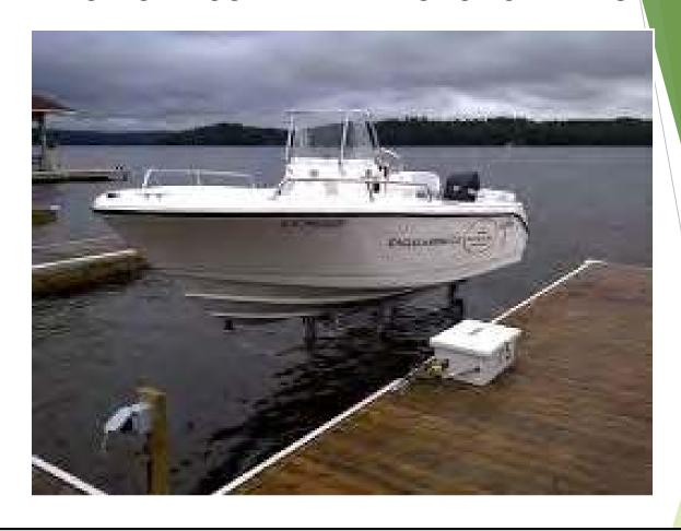
Canal bottom mounted hydraulic lifts are hydraulic scissor jacks with bunks to support the vessel. These lifts can be operated with either water supplied by hoses, or with oil pressurized by pumps. These lifts are very difficult to inspect because the majority of the lift is underwater all the time. I do not inspect these lifts, I make note of it and recommend consultation with a specialist.
