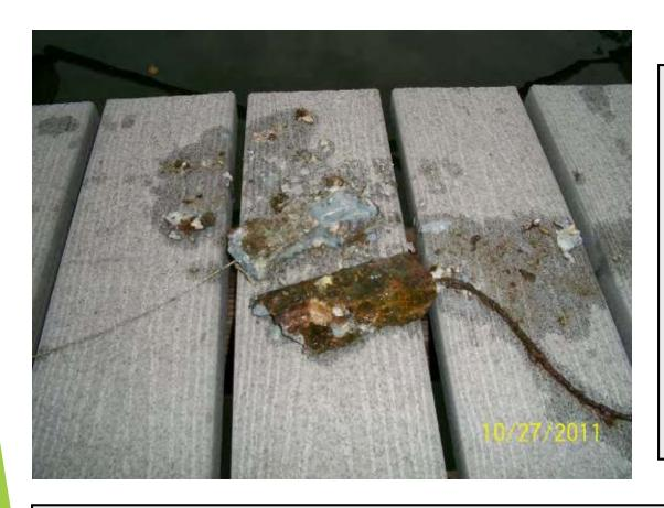
For best results zincs should be suspended within the water column, not resting on the bottom or in contact with the lift structure. Try to determine that the zincs will not be left high and dry during low tide. You also want to make sure that the zinc cable is connected to the lift structure not the dock.
