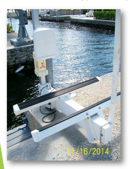
The most common type of personal watercraft lifts are the "Up & Over" type which lift the vessel UP and then rotate the watercraft OVER onto the land or dock surface to allow access and servicing.
