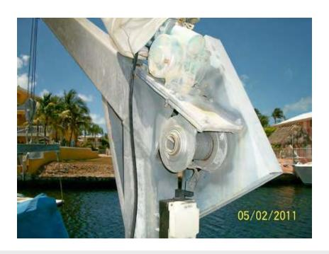
Davits and boat lifts have many components that are common to both. With the exception of hydraulic side elevator lifts, all davits and lifts have cables and typically winder spools or winder bars. Davits and lifts also have motors that drive either a belt/pulley or a housed direct drive gear. And obviously, davits and boat lifts have similar switching and wiring. In the next few slides we will discuss inspecting these common components.
