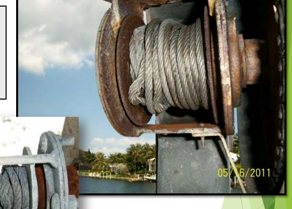
In both of these cases you would report that the damaged cables need to be replaced.
