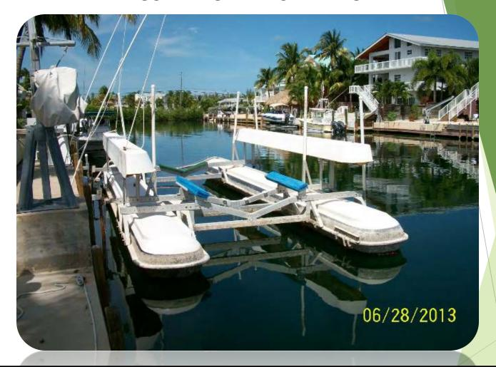
Submersible boat lifts are designed to float with the vessel out of the water, then submerge when launching the boat. These lifts can be VERY difficult to inspect and test. They do not want to submerge when there is not a boat on the lift. I do not inspect these lifts, I make note of it and recommend consultation with a specialist.
